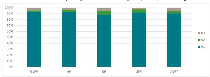
Figure 1: Relative contribution by life cycle stage for 1 metric ton of fabricated HSS
